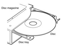
• The disc tray may be taken off from the magazine if you pull the tray forcibly. If the tray is taken out, put it back into the magazine as illustrated. Be sure that both ends of the tray are aligned to the grooves of the magazine correctly.
